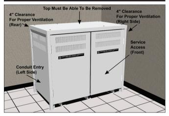
B 37.5 - 150 kVA Single Phase Series 900 45 - 150 kVA Three Phase Series 900 15 - 75 kVA Three Phase Series 900/200 37.5 - 150 kVA Single Phase Series 900/200
