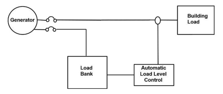
The Automatic Load Level Controller adds and subtracts Load Bank load in response to dynamic power fluctuations in the connected facility load. It utilizes the Load Bank as a "supplemental load" for maintaining a minimum load on the power source.
