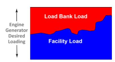
The Controller will continue to add & subtract load in response to the power fluctuations of the connected building load. By maintaining a minimum load on the power source, the various low load issues like Wet-Stacking are eliminated.
