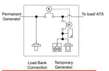
Dual purpose dual breaker with male & female camloks to connect a load bank or temporary power sourceIncludes main breaker for the temporary load and permanent line connections.
