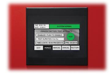
The color touchscreen display on the Intellistat TS provides all electical parameters, inverter status, programmable inverter and battery testing, and data-logging. Optional Intellistat TS communications allow for remote monitoring and reporting via BACnet/IP or BACnet MS/TP, Ethernet TCP/IP, MODBUS TCP, or MODBUS RS485. For more details, see the Network Communications description on Page 7.
