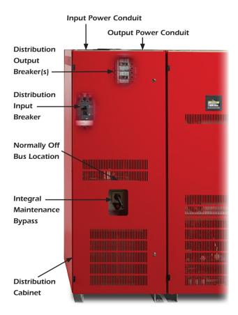
**NOTE:** Distribution Cabinet is optional with NNX models, but standard with LLX, NLX, VVX, and VLX models. Input and output transformers required for these models are located within the Distribution Cabinet.
