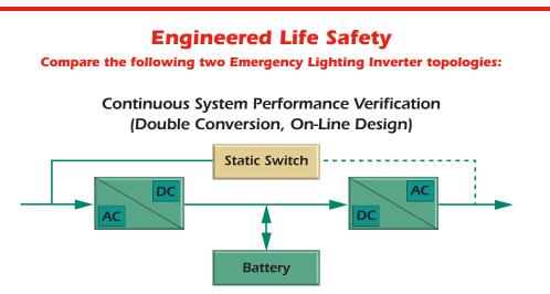
System performance is ensured, system continually self-checks 24 hours / day; 7 days / week. Provides clean, conditioned and regulated power to LED drivers and electronic ballasts that are being utilized for egress lighting.
