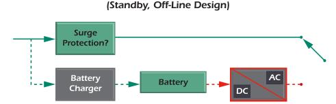
System performance is verified under only two conditions: 1) if / when it is periodically tested, and 2) during an emergency. MAY NOT provide surge protection, and DOES NOT provide power conditioning or regulated voltage to LED drivers and electronic ballasts that are being utilized for egress lighting. Inverters promoting 98+ % efficiency are typically off-line or standby designs, or "operating" in a bypass / standby mode.
