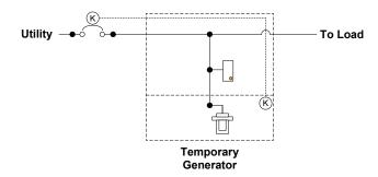
Generator Docking Station with male Camloks behind a Kirk Key door interlocked with an existing circuit breaker, includes pass thru lugs to land permanent line connections
