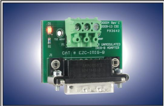
The Cyber Sciences' EZ Connector for IRIG-B (EZC-IRIG-B) or DCF77 (EZC-DCF77) is a wiring adapter for the CyTime™ Sequence of Events Recorder (SER) to facilitate wiring of its precision time-sync input signal. The adapter fits the “Options” port (DB15 connector) of the SER and facilitates wiring of IRIG-B or DCF77 signals via a screw-type terminal, suitable for power equipment wiring. (Model EZC-IRIG-B is shown at left.)
