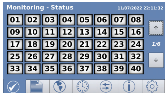
Figure 4-1. Monitoring status screen. (SER-32e) Image shows one additional Input Module added (Inputs: 33-40).
