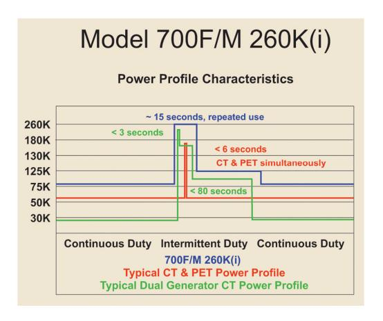
**Note:** The illustration above is a typical medical equipment power profile that depicts the proper application of a K(i) rated power conditioner or voltage regulator.
