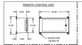
RESISTOR COMPARTMENT HAS A SCREENED TOP AND SOLID SIDES (OPEN BOTTOM). INSTALL RESISTOR ELEMENT SECTION OVER GENERATOR EXHAUST VENT
