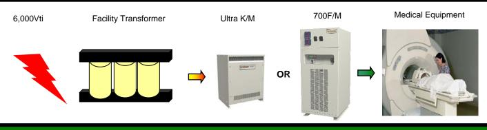
Ensures Maximum let through voltage of 330Vp (on 208V) when exposed to a 6,000V / 3,000A waveform
