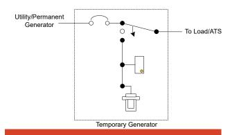
Service entrance rated TMTS with 3 position rotary to transfer between utility and temporary source
