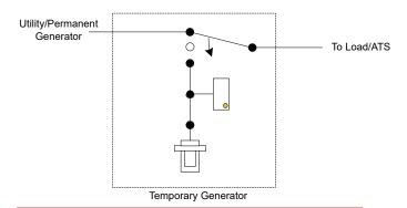
Base TMTS with 3 position rotary to transfer between permanent and temporary source
