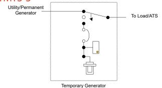
TMTS with temporary generator breaker to allow transfer between permanent and temporary source
