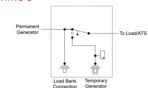
Dual purpose to allow load banking of permanent generator and connection of temporary source
