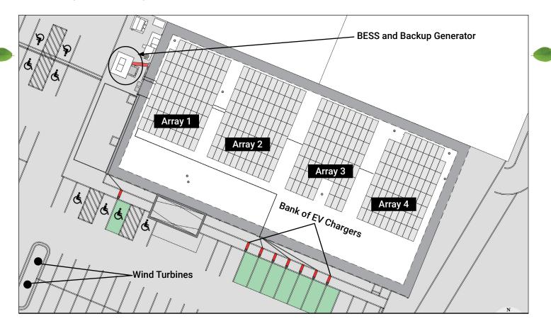
Solar arrays 1-4 are on the roof of the cafeteria portion of the facility and generate 172.8kW of combined potential output.
