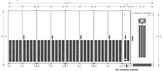
A field-installed DC Landing Cabinet is included whenever (3) or (4) battery cabinets are provided, and is reflected in the dimensions of Configurations C and D above. The DC cable connections from each battery cabinet's circuit breaker are landed on the positive and negative bus bars within the landing cabinet. A single DC connection is then made from the landing cabinet to the inverter's DC input.
