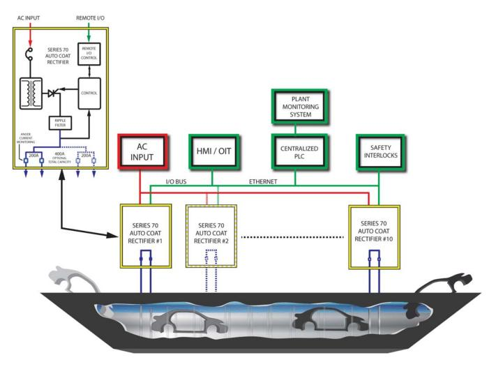
For the sake of illustration, we have only shown (10) ten rectifiers, each powering (2) two anodes. (Note that most automotive continuous conveyor e-coat lines will have more than (10) rectifiers.) Hard-wired safety interlocks are not shown here, but note that they are available.
