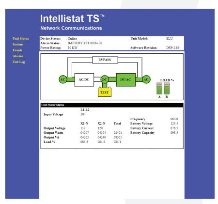
Example of a "Model ELU" inverter "Unit Status" screen, via the "Intellistat TS" web-based network communications.
