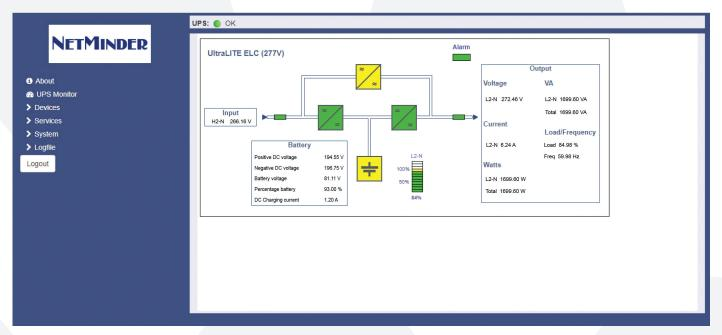
Example of a NetMinder inverter monitoring screen, via the adapter's internal web interface.
