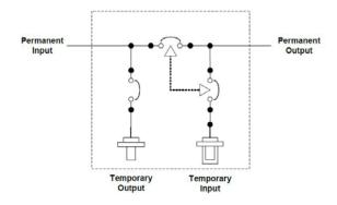
Dual Purpose with permanent generator, temporary generator and load bank overcurrent protection.
