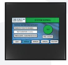
The color touchscreen display on the Intellistat TS provides all electrical parameters, inverter status, programmable inverter and battery testing, and data-logging. Optional Intellistat TS communications allow for remote monitoring and reporting. For more details, see the "Optional Network Communications" description on Page 7.
