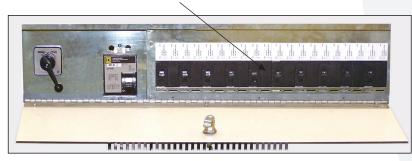
Hinged, key-lockable, drop-down panel allows front access to standard input breaker, inverter bypass switch, and optional output distribution circuit breakers.
