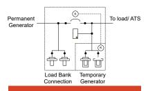
Dual purpose single breaker docking station with male and female camloks to connect a load bank and temporary power source.
