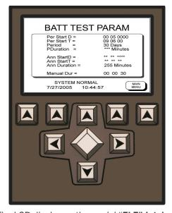
The LCD display on the model "ELE" <u>Intellistat</u> provides all electrical parameters, inverter status, programmable inverter and battery testing, remote monitoring and reporting, and data logging. An optional integrated fax modem can be included in the closed-loop communications system.
