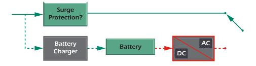
System performance is verified under only two conditions: 1) if / when it is periodically tested, and 2) during an emergency. MAY NOT provide surge protection, and DOES NOT provide power conditioning or regulated voltage to LED drivers and electronic ballasts that are being utilized for egress lighting. Inverters promoting 98+ % efficiency are typically off-line or standby designs, or "operating" in a bypass / standby mode.
