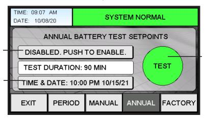
Press the "TEST" button to invoke a battery test \* (Duration is dependant on battery option purchased). The duration is preset at the factory and is not user accessible. Contact the factory should the duration time need to be modified.
