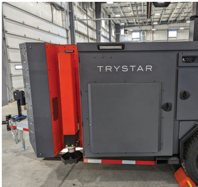
LP Tank Storage Cabinet Door
