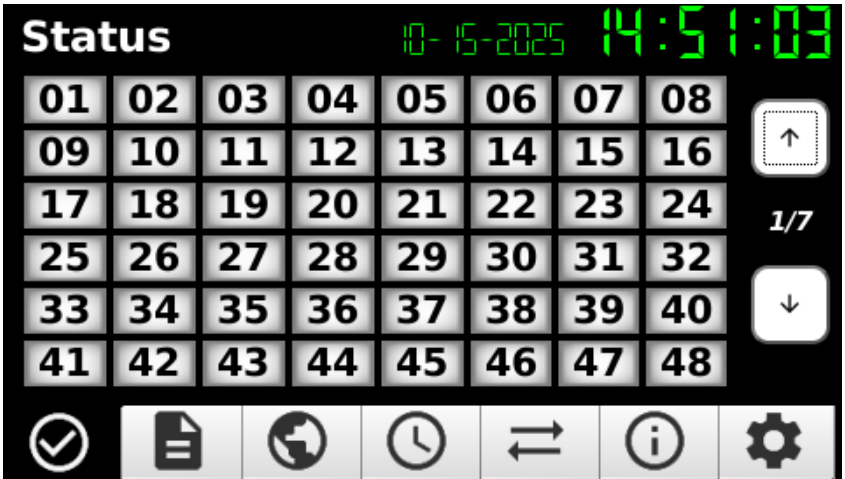
Figure 4-1. Monitoring - (on SER) Status screen.
