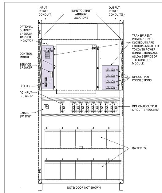
Bypass Switch, AC Input Breaker, and Optional Output Circuit Breakers are located behind a hinged, key-lockable, drop-down panel door.
