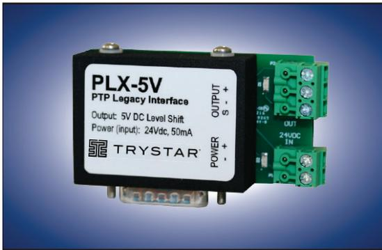
**Note:** The specific PLX model (PLX-5V or PLX-24V) determines the output signal's nominal voltage: 5 Vdc or 24 Vdc, respectively. The output protocol (IRIG-B, DCF77 or 1per10) depends on the time-sync output setting configured for the master Trystar SER-3200/2408 Event Recorder.
