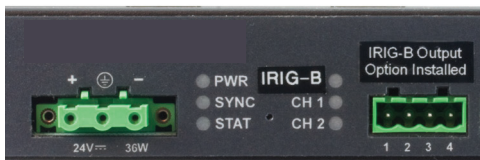
STR-100/IRIG-B front view (close-up)
