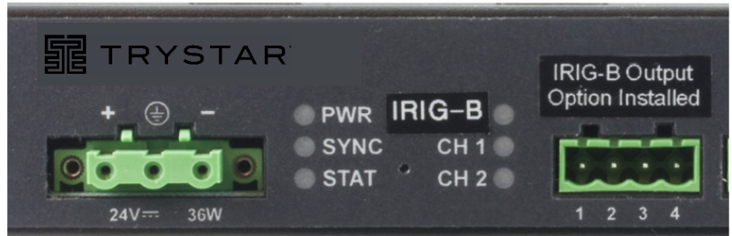
STR-100/IRIG-B front view (close-up)
